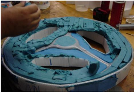
Once the Plat 55 has cured, flip the mold over, remove the mold base, and begin digging all of the clay off of wheel. DO NOT remove the wheel from the poured silicone rubber mold. The seal between the mold and wheel is critical in producing a smooth/clean seam line. A putty knife and/or Alumilite Spatula tools are helpful in removing clay around and near steering wheel.
