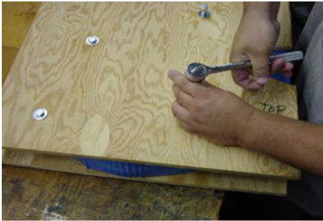
The bolt holes will line up with the holes in the mold left to take up space and will not interfere or touch the silicone at all.
