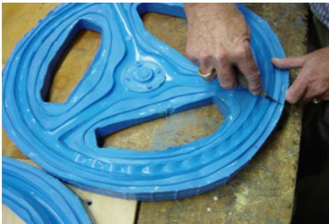
Using a Key Knife or Excel blade, cut a wedge in the mold to produce a pour hole for the resin. For cosmetic reasons cut the half of the mold that will be the back of the steering wheel.
