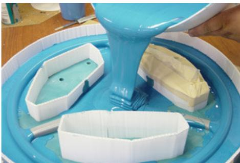
Once the critical detailed surface is covered, begin pouring the bulk of the rubber in the center of the mold box allowing the silicone to flow naturally over the part until it completely covers the wheel.
