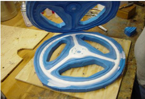
The mold will separate and you will find your cast steering wheel with minimal flash and a small seam line around the pour hole section on the back of the part that can easily be cleaned up.
