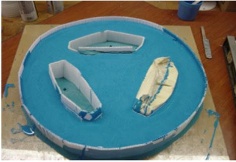
Make sure the liquid rubber covers the part by at least 1/4"-3/8" and make sure your mold box and inside cavities are not leaking. Allow the rubber to cure overnight.
