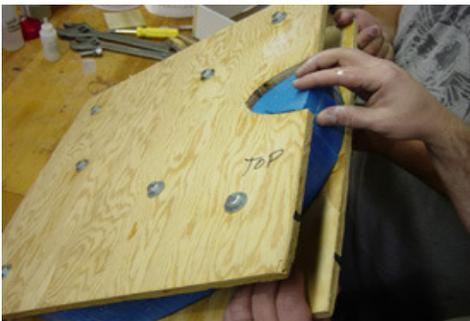
Once the mold is full, place the pour hole cut out back into its position which will squish out the excess resin and fill the detail back into that section of the steering wheel.
