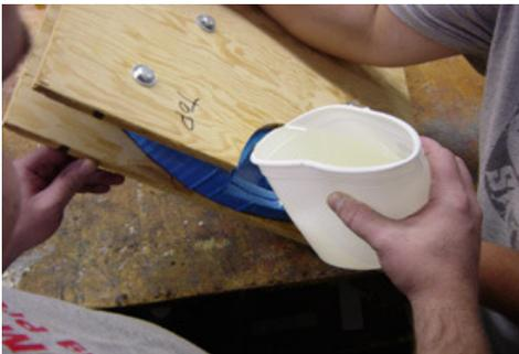
An extra set of hands may be necessary depending on the size of the mold. Continue to rotate the mold back and forth until the mold is full of resin.
