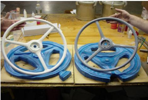
You now have an exact replacement for your antique car steering wheel. The mold is ready to be put back together and poured again.
