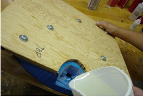
While pouring, tilt the mold to help the resin flow into the different areas in the mold and to eliminate undercut areas which will allow any air bubbles to flow back up to the pour hole and escape.
