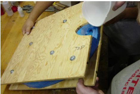
Tilt the mold to allow the resin to flow down the side of the mold to decrease the chance of creating air bubbles when pouring. Pour slowly to allow the resin to flow naturally into the mold.
