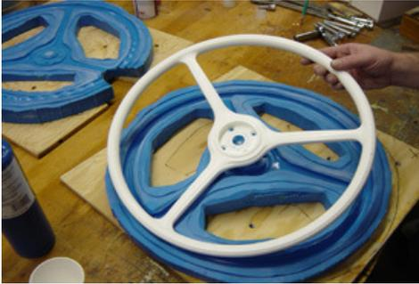
Remove the steering wheel from the mold and with your fingers or a dull knife remove any excess flash.
