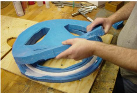
Once the resin has cured, remove the bolts and boards supporting the mold and begin to separate the two halves. Continue to work around the outside edge to separate the two halves.
