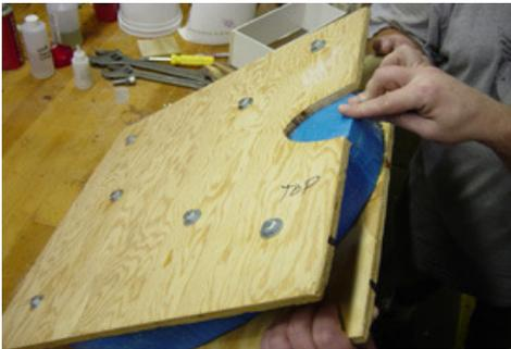
Press the cut out section firmly back into place until the U channel made by the Key Knife snaps into place.
