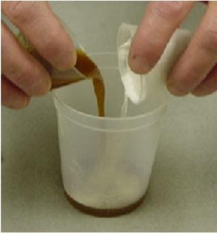
Mix equal amounts of each side of the resin with the same amount of microballoons (the 'B' side is being shown in the picture). Repeat this process for the 'A' side.
