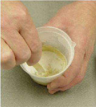
Stir in the microballons until uniform color is reached. Since you are mixing a substance into the Alumilite, keep in mind that you are also thickening the Alumilite. When you eventually mix the two sides together and pour the microballoon filled resin into your mold, the consistency or viscosity will be a little thicker.
