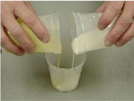
Pour both sides of the Alumilite Casting Resin with microballoons into a cup.
