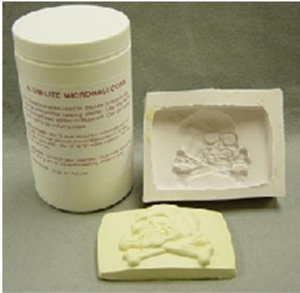
Once the casting resin has hardened and cured, demold your cast piece. Your cast replica will have the exact detail of your original with the characteristics of the filler you used.
