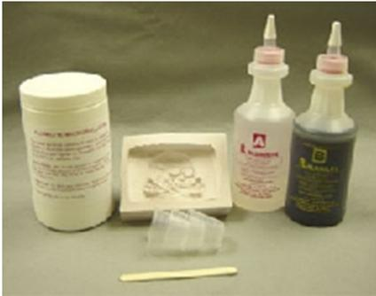
The first step is to gather the materials that are needed. Alumilite Casting Resin, a stir stick, cups, filler (we are using microballoons), and your mold.
