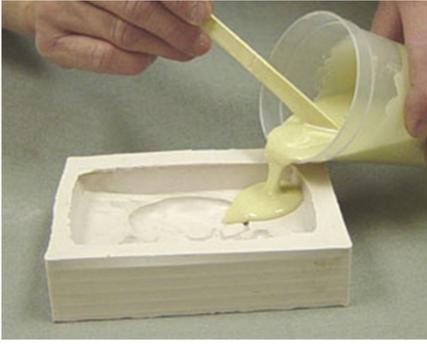
Slowly pour resin into your mold. Remember, you can tip the mold a little while you pour to help fill in any undercuts and reduce the chance of air bubbles.
