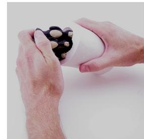
6. Once the mold has been removed from the mold box, flex the cured silicone mold and remove your original. You now have a perfect mold of your unharmed original. You are now ready to make identical castings of your original.
