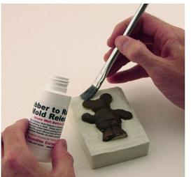
Once you have completely removed the clay, coat the rubber with Alumilite's Rubber to Rubber Mold Release. This will prevent the second layer of silicone rubber from adhering to the first. Vaseline works great for this if you do not have any of rubber to rubber release. **DO NOT MOLD RELEASE THE ORIGINAL** and be sure not to miss any rubber sections of your mold. Any area not coated with release agent will stick and will require cutting to separate the two halves apart.
