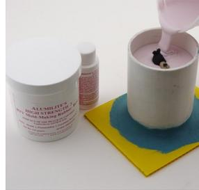
4. Measure and mix the silicone rubber according to the instructions provided with the silicone. Once mixed thoroughly, slowly pour the rubber from one corner of your mold box allowing the silicone to flow naturally around your piece. (we have chosen to use High Strength 2 due to the large undercuts - bear's chins)
