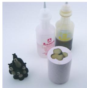
3. The open time of most Alumilite resins is 90 seconds. The color change is the end of the open time and the point in which it begins setting up. The finished color of Alumilite Regular is an opaque tan (white and black resin is available along with coloring dyes to color the resin yourself).
