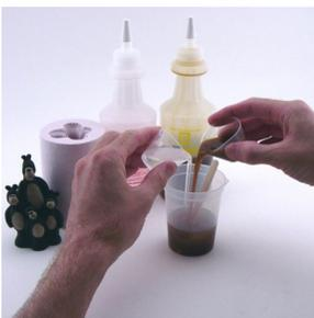
1. Measure the Alumilite resins according to their proper mix ratio (generally 1:1 by wt or volume). Mix vigorously for 20-25 seconds until thoroughly mixed.
