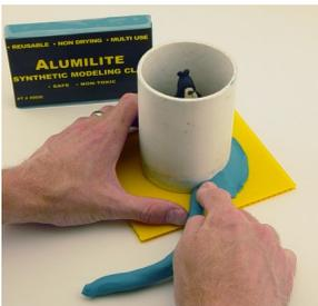
3. Make a mold box out of plastic, wood, metal, posterboard, pvc, or any other cup or container. Leave .25"-.375" between your mold box and your original. Seal your mold box with Alumilite's Synthetic Modeling Clay to prevent the mixed silicone rubber from leaking out of your mold box before it cures.
