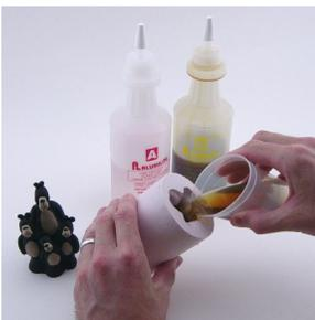
2. Once you've mixed the material thoroughly by scraping the sides and the bottom, slowly pour the resin into your warm mold by tilting it and letting the resin flow down the sides of the mold. Squeeze and tap the mold to assist any unwilling air bubbles to release from the sides of the mold and to help them float to the surface.
