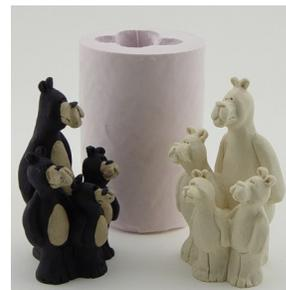
4. Once the resin has hardened (approx. 5 minutes), flex the mold and remove your perfectly cast piece. Your piece is now ready to be sanded, painted, tapped, machined, etc.
