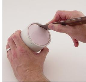
5. Let the rubber cure (typically takes overnight). Once the rubber has hardened, begin demolding the original. If you can not disassemble the box itself, use a dull knife or spatula to remove the mold. Rubbing alcohol helps by releasing the surface tension and making the silicone slippery.
