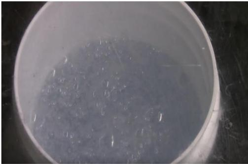
**Vacuum Degassing (if available):** Once Amazing Clear Cast has been thoroughly mixed, if you have vacuum degassing equipment, we recommend degassing prior to pouring to minimize air bubbles. If you do not have this equipment, proceed to next step.
