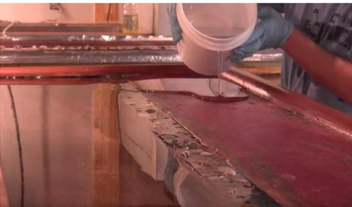
**Application thicknesses greater than 3/8" in a single pour may shrink, discolor, pull away from surfaces, and/or warp.** Where thicker coatings are desired, it is recommended to pour multiple coats. Additional coats can be applied no sooner than 3-4 hours and no longer than 12 hours for optimum adhesion.
