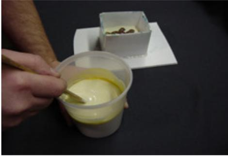
Measure and mix the proper amount of silicone required to fill the second half of the mold. Once again, if you need help calculating the volume needed for your piece, visit the [Material Calculator](#) page on our website.
