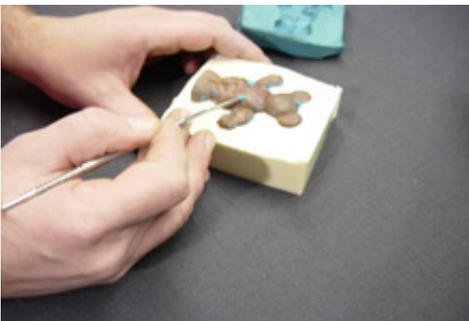
Using your Alumilite clay tools, remove every tiny bit of clay from the mold and original.
