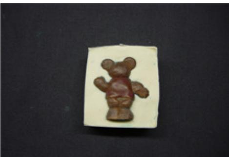
Once you have cleaned the mold and master off completely of all clay residue, you are ready to cut your locators so the second half of the mold aligns with the first.
