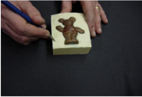
Using an Excel knife or better yet a U-Channel knife, cut "v" or "u" channels in the rubber mold. This will allow the rubber you pour during the second half to flow into these channels and provide great locators to align the two halves of the mold.
