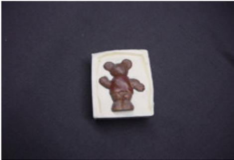
Cut locators on at least two or three sides of the mold.
