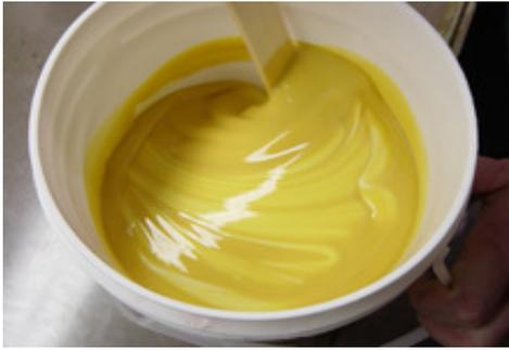
A very easy to use, general purpose, 2 part silicone mold making rubber is Alumilite's QuickSet silicone. It has a very low viscosity, picks up great detail, and is great for simple one and two piece molds . Using the cups and scoop inside the QuickSet kit or by measuring the mix ratio of 10 parts base to 1 part catalyst, properly measure the QuickSet and thoroughly mix the rubber. If you need help calculating the volume needed for your piece, visit the Material Calculator page on this site.
