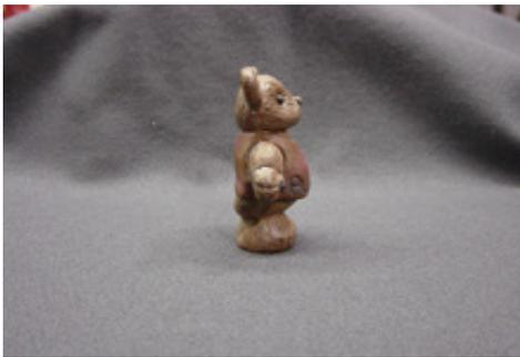
As you can see with this bear, the back is not flat and has detail in which the mold and casting will need to have in order to reproduce the piece exactly. In order to mold both halves, you will need to start by making a mold of the front and then making a mold of the back. You will need to start by determining a parting line which is where the two halves of the mold will meet. This is typically an edge or perhaps the half way point from the front and back.
