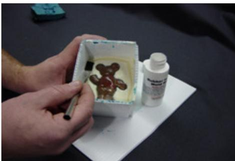
The other option is to use Alumilite's Rubber to Rubber Mold Release. Shake the bottle well before using and brush on multiple coats waiting 5-10 minutes between coats before applying the next.
