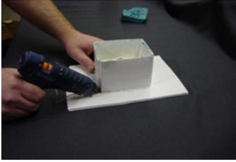
Before pouring your second half of your silicone rubber mold, be sure to check that your mold box is sealed and seal any gaps you may find to eliminate the chance of your entire silicone batch leaking out a hole in your mold box. Once the silicone starts to leak, it is nearly impossible to stop and creates a huge mess along with wasted time and material. It is always best to take a minute to double check to make it is sealed well.
