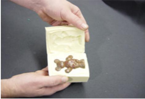
As you can see, the mold will separate exactly where the two halves were poured and mold released. You will also see how the second half of the mold filled in the locators from the first half and how it will give you perfect alignment between the two halves.
