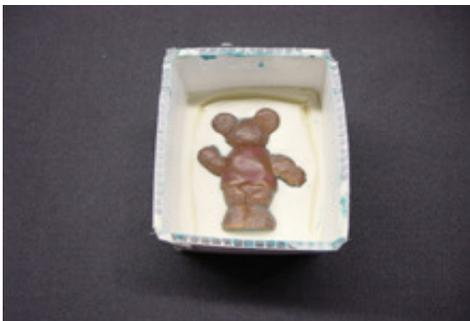
Place your mold back into the mold box and reseal it if necessary.
