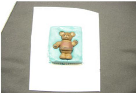
Once the part is completely clayed up to the parting line you've established, you are ready to build your mold box to contain the liquid rubber.
