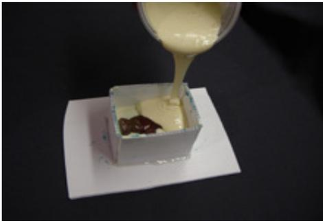
As you did with the first half of the mold, pour the rubber from one corner of the mold box and allow the material to flow naturally over your original and cover it by at least  $\frac{1}{4}$ ".
