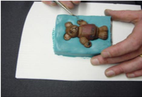
Using clay tools, smooth and flatten the clay to establish a perfectly smooth and clean parting line where the clay touches the part. The cleaner the edge, the smaller your parting line will be and the less clean up will be required on the seam line of your cast resin piece.
