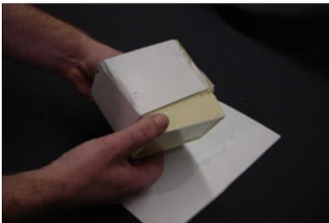
Remove the mold from the mold box.
