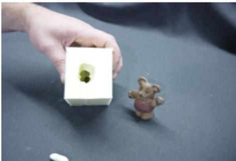
Once you have both channels cut out and place the mold together, you will find a perfect pour hole in which you are ready to pour an exact replica of your original. You can also use 1/8" copper or brass tubing to twist and cut holes through the silicone to place vents and/or injection points throughout the mold.
