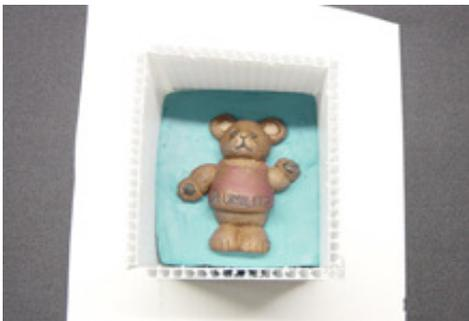
Using corrugated plastic, angle iron, wood, a recycled piece of plastic, Legos, or any other non porous material, construct a mold box to contain the liquid silicone rubber. Build your box so that the walls are  $\frac{1}{4}$ "- $\frac{3}{8}$ " around the outside of your original. Building your walls too big around the outside of your piece require much more silicone which wastes unneeded silicone.
