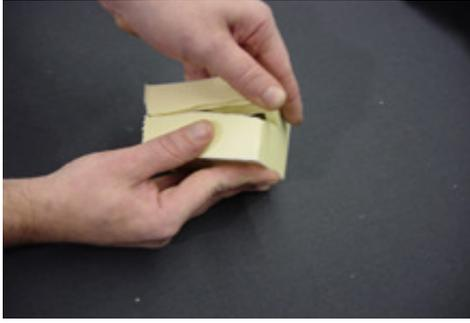
Using your hands, find the seam line and begin to separate the two halves of the mold.
