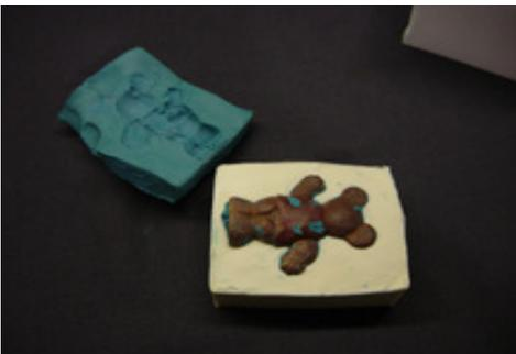
Remove the bulk of the clay and then go back and clean off all of the left over clay.
