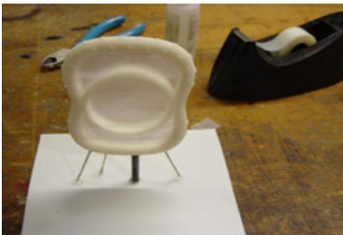
Once the supports are glued and trimmed to the proper size, glue the supports to your mold base using super glue or a small amount of hotmelt.
