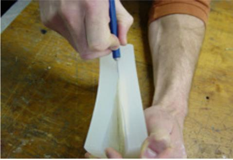
Continue cutting around the part being careful not to put too much pressure on the part that would damage it. Some small scratches on the original may be unavoidable.
