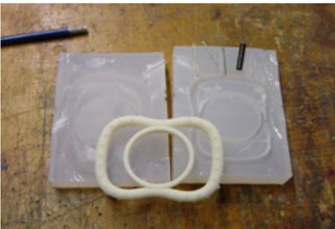
Remove the tape from the inside flange area and remove your piece as well as your vents and gates.
