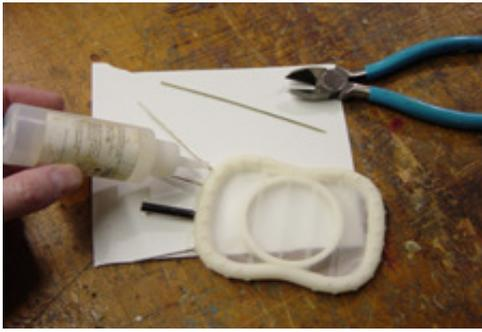
You are now ready to glue on wire, wood, or plastic tubing to your piece to act as supports for suspending but also to act as pour and vent holes in your finished silicone rubber mold.
