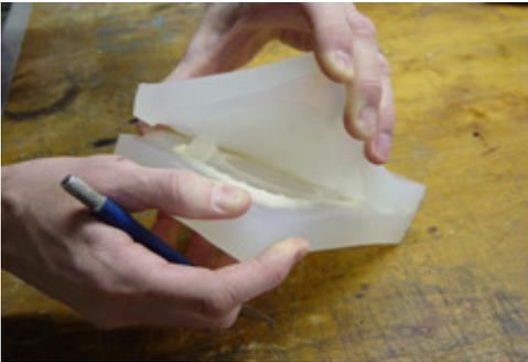
As you cut to the part, the tape will separate the inside portion of the mold and provide you with a perfectly smooth and crisp parting line.
