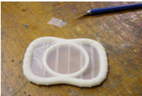
Continue trimming the excess tape off until the entire piece is neatly trimmed. If your tape hangs out away from your original, you must color the cellophane tape with a permanent marker in order for you to see the tape in the cured silicone rubber mold. This will allow you to find the tape edge and cut directly to the tape. In this example, the tape is on the inside edge and we will be cutting to the part and therefore did not need to color the tape.
