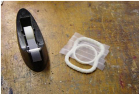
Begin by making sure your master has the surface quality and finish you desire in your finished part as well as making sure your master is free and clean of any dust, dirt, oil, or grease. Then using cellophane tape, begin taping and overlapping the tape where you have determined the best place to establish your parting line.
