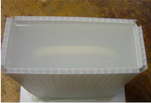
Allow the silicone to fully cure before demolding. Standard demold times are overnight at room temperature.
