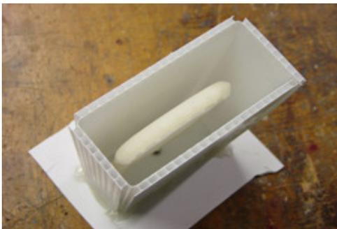
Build your mold box to contain the liquid silicone rubber. Seal the mold box extremely well to prevent the silicone from leaking.
