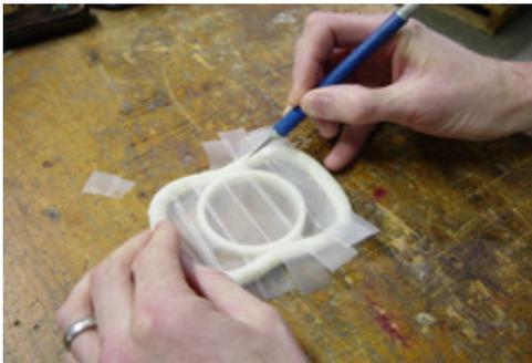
Once you have the parting line completely taped off, using an Excel Knife, trim off the excess. Cut the tape as close as you can to where the tape comes in contact with the part to avoid excess thickness in your casting that would have to be sanded down or finished after being cast.
