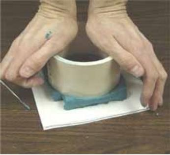
Use a section of PVC pipe or another mold box material such as Corrugated Plastic, recycled plastic container, or metal ring that is approximately 1" in diameter more than the lens. Press the PVC down around the lens. This will serve as your mold box. This will leave approximately 1/2" around the outside of your lens.
