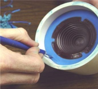
Once you have removed all of the clay, use an Exacto knife and cut some "V" shaped wedges in the outside flange area (rubber between the lens and the mold box). You can also use Alumilite Carving Tools to cut U-shaped grooves into the silicone.
