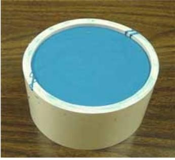
Allow the material to cure. The Plat 55 demold time is approximately 8 hours at room temp. Temperature will affect the cure rate. The warmer the temperature, the faster it will cure. The warm temperature will also reduce your work/open time.
