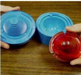
Once the two halves fully separate, remove your original. You are now ready to begin pouring duplicate lenses using Alumilite's clear resins.
