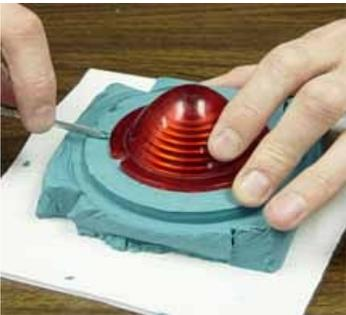
Remove the PVC tube from the clay. Press the lens down into the bed of clay and using Alumilite's clay tools, begin smoothing out the clay which will create your seam line between the two halves of the mold. Take your time and make the edge where the clay touches the lens very neat and clean. The cleaner the clay line, the smaller your flash will be on your finished cast lens.
