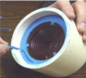
Then peel or pull away the rubber so you have a small groove in the cured rubber. These will act as locators to line up the two halves of the rubber.
