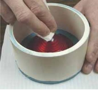
The last thing you want to do is to clean the lens before pouring the rubber. Use some rubbing alcohol and some paper towel to gently clean all fingerprints and clay off of the lens.
