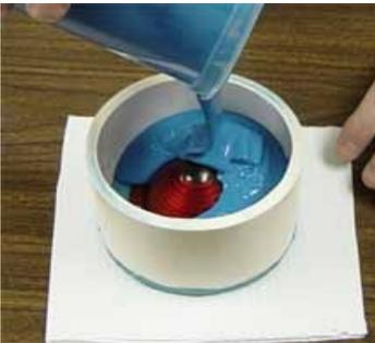
Once the rubber has risen and fallen, allow it to bubble under full vacuum for another 1-2 minutes. Then remove the degassed Plat 55 and simply pour the rubber in a corner of the mold box which will cover the lens. We recommend the lens to be covered by at least 1/4" inch of rubber which will be the depth of your mold over the top of the lens.
