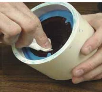
Before pouring the second half of the silicone rubber, make sure to clean the lens one last time to make sure there is no clay or other contaminants on the surface of the lens.
