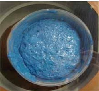
Place the rubber in the vacuum chamber and allow the liquid rubber to grow until it collapses on its own.
