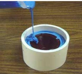
Once you have effectively degassed the rubber, slowly pour the second half of the mold allowing the rubber to flow from one side of the mold on its own. Do not dump the material in but rather pour from one spot and allow the material to flow naturally.
