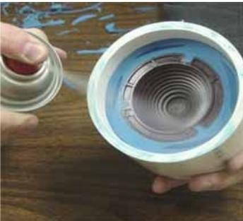
Next mold release the rubber using Alumilite's UMR. Silicone rubber will stick to cured silicone rubber and therefore needs to be released. Simply spray on a thin layer where ever the next pour of liquid silicone will be in contact with the first half of the mold that is already cured.
