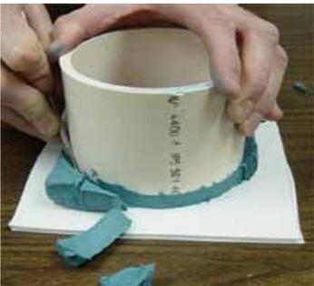
Once you have the clay line as good as you can get it, press the PVC tube back over your lens and into the clay. Then trim the excess clay away from the PVC which will serve as your mold box.
