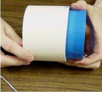
Once the rubber has cured, break the tension between the outside edge of the rubber mold and the mold box and push the rubber mold out of the PVC. Rubbing alcohol works to help release the rubber mold from the PVC pipe. Simply squirt a little down the gap and use a dull knife or Alumilite Spatula tool to break the surface tension between the two and easily remove the rubber mold.
