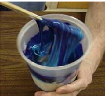
Once you've added the catalyst, mix it thoroughly until every swirl on the container wall and throughout the rubber is gone. The Plat 55 has a 90 minute work time so you have plenty of time to mix it thoroughly and vacuum it.
