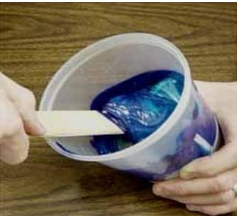
Mix the rubber thoroughly. Make sure the sides have been scraped and that there are absolutely not swirls in the liquid rubber.
