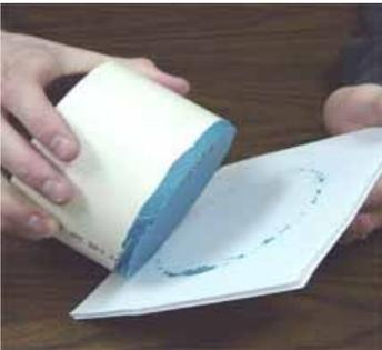
Once the silicone rubber has cured (typically takes 8 hours at room temp for the Plat 55), remove the mold from the plastic base.
