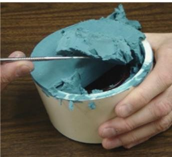
Using Alumilite's clay tools, dig out all of the clay away from the second half of the mold.
