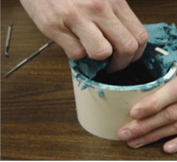
Remove every little piece of the clay and **BE SURE NOT TO REMOVE THE LENS FROM THE MOLD OR THE PVC TUBE**. You do **NOT** want to break the seal between the lens and the rubber mold you just poured! Nor do you want to break the seal between the mold and the PVC tube.
