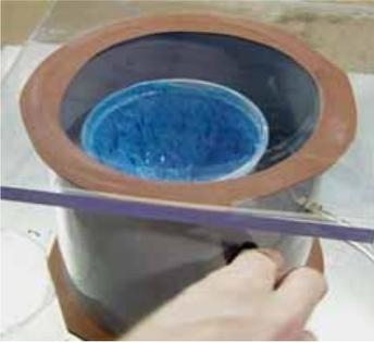
Here you can see the material sagging back down the walls of the container after the material has risen, crested, and fallen. Keep your hand on the release valve to allow atmospheric pressure back in the chamber if the rubber is going to rise up over the top of the container.
