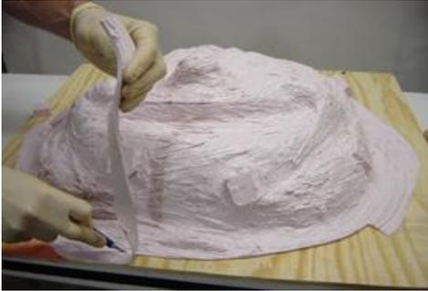
When the silicone cures, trim the excess flange area off with a knife. This will make a cleaner and straighter flange for the mother mold to mate to.
