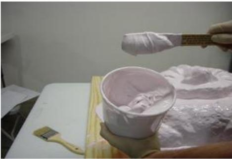
Continue this process until you achieve your desired consistency of the rubber that will allow you to paint on and build up your silicone rubber wall thickness.
