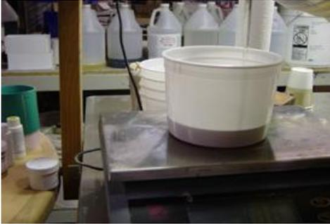
Mix equal amounts of the Alumilite Shell Casting Resin A and B side and immediately start to mix.
