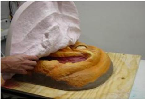
With some pieces, it may be difficult to remove the rigid mother mold from the original without first peeling the silicone rubber from the original to release the surface tension. Therefore, work the silicone up around the edges and peel it up off of the original on one side and then the other.
