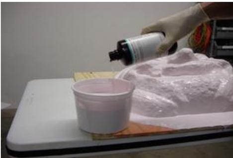
For your next step mix up approximately double your first coat and now add some Alumilite Thixotropic Additive to make the consistency of the rubber thicker. This will enable you to paint on a thicker layer of silicone to build up your wall thickness of your mold. Start by adding only a few drops of the Thixotropic Additive to the mixed silicone rubber. This will only make the mixed rubber thicker and does NOT affect the work or cure time of the rubber.
