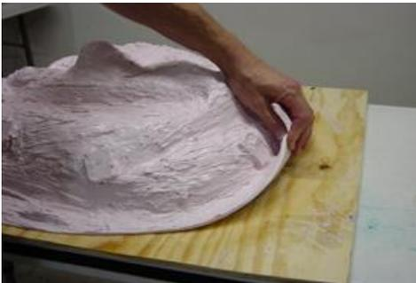
Then simply lay it back down into place over the original. Make sure all sides are released. This will make the removal of the rigid mother mold much easier.
