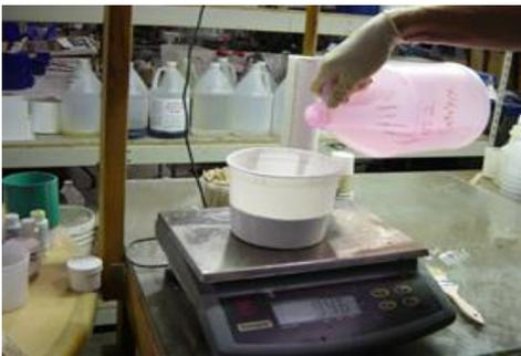
We used approximately 1.5 lbs of base and .15 lbs of catalyst to paint on our initial skin coat. The High Strength 2 has a mix ratio of 10:1 by weight.
