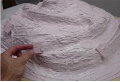
As soon as you are done painting on your build up layer, place some locators (here we used some small cut up sections of old High Strength 2 rubber molds) on the back side so the mother mold will properly line up with the silicone brush on mold. You can use glass marbles in place of the chunks of silicone if needed.
