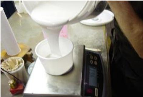
The initial coat of our silicone rubber will be straight High Strength 2 mold making rubber from Alumilite. This silicone is a flexible rubber with great tear strength.
