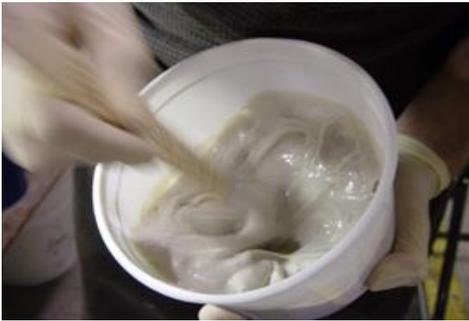
Within 30 seconds of the two parts coming in contact with one another, the material will start to thicken. As it thickens, it is not curing but rather building thickness to a brushable consistency.
