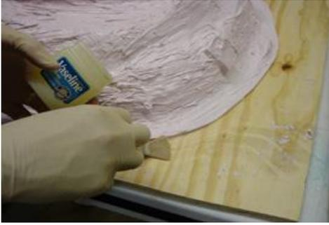
It is a good idea to seal the wood base where the Shell resin will come in contact with Vaseline to ensure an easy release.
