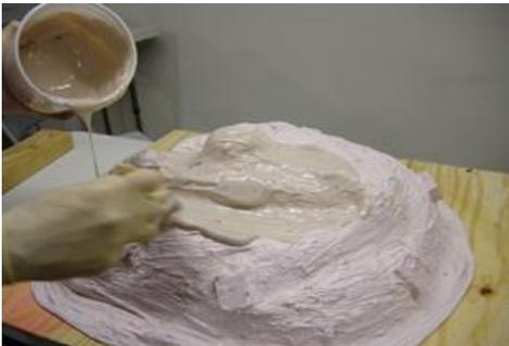
You are now ready to start brushing a coat of Shell over the silicone mold. Be sure to cover the entire area evenly. We used two coats of approximately 3 lbs each to cover and complete the mother mold. Be sure to only mix enough material that you can work with in the 7 minute open time allowed.
