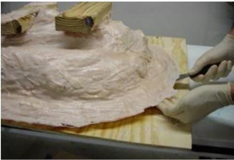
Once the Shell resin has cured, using a putty knife, pop the mold and part off of the wood base.
