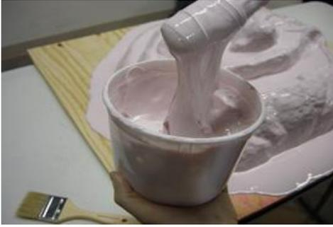
The recommended percentage is .5% Thixotropic Additive which is difficult to measure. Therefore start with a few drops, mix it, and evaluate the consistency.
