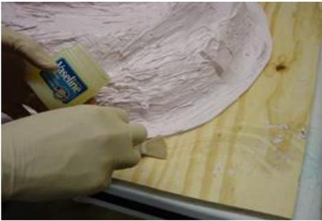
In this How To we are going to demonstrate the process of making a brush on mold using Alumilite's High Strength 2 silicone rubber and a rigid mother mold using Alumilite's Shell Casting Resin for a quick and cost effective alternative to pouring block molds. We will then show you how to make beautiful hollowed out cast replicas. Here we are making a mold of a paper mache hand sculpted decorative pumpkin that can be hung either indoors or outdoors.
