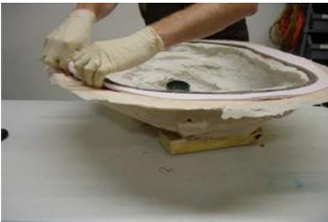
Begin working the edge around the mold and part to release the mold from the original.
