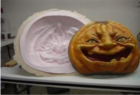
You should be able to remove the original with very little damage. The silicone will not affect the paint or any part of the original as long as the original is not porous and does not allow the liquid silicone to soak into the surface of the original.
