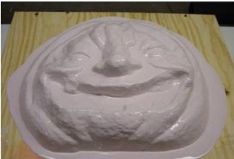
Continue to paint on the initial thin coat of rubber until the entire piece and 1-2" of flange area is covered.
