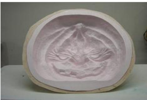
The silicone brush on mold and mother mold are now ready to start producing parts.
