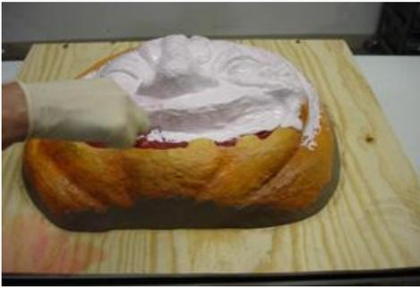
Work the silicone into the detail of the master with the brush, making sure every bit of detail is coated with a thin layer of rubber. This initial coat ensures the detail is picked up in the rubber mold. The next steps are to add thixotropic additives to the following coat/s to build thickness behind the initial thin coat which will add durability and toughness to the paint on rubber mold.
