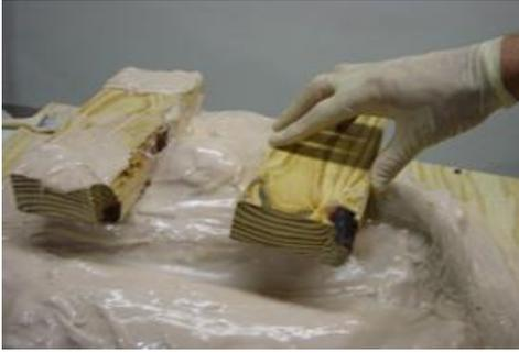
Before the material cures, set and paint in a couple of wood blocks that can be used as a stand or mounting area.
