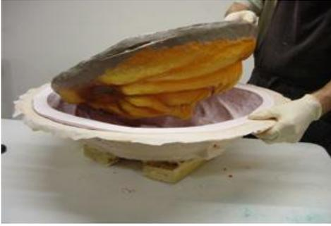
Once you've worked the part loose, simply pull the original out of the rubber mold. This will be fairly easy since you've already peeled the silicone off of the original before painting the Skin Coat on.
