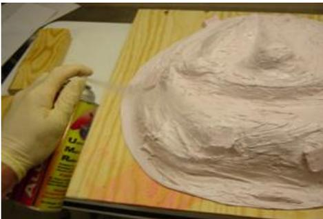
Before painting on a coat of the Shell resin to make your mother mold, spray the UMR to allow for an easier release between the silicone brush on mold and the rigid mother mold. You can also use Stoner Mold Release if available.
