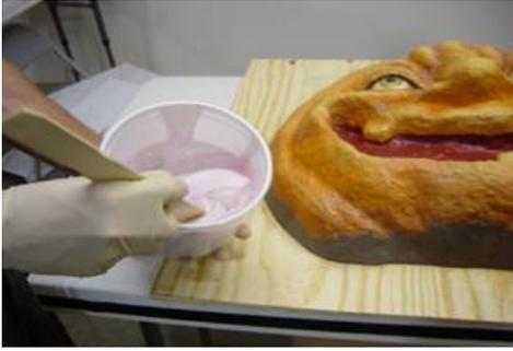
Mix the rubber thoroughly until absolutely no swirls are seen in the rubber or along the sidewalls of the bucket.
