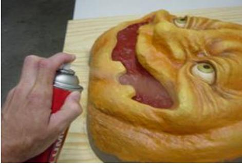
Using Alumilite's UMR release, spray the mold and wood to ensure a good release.
