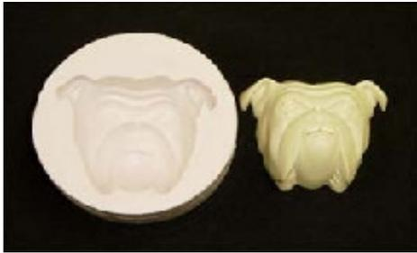
A one piece mold works perfectly for parts like this bulldog that have a flat back side. The flat back side gives you a noncosmetic side to pour from. The advantages of a one piece mold are the simplicity of making the mold and no seam lines in your finished casting. This particular bulldog was used for as part of a beer tap found in bars across the country. This How To process will walk you through the steps for making this one piece mold.
