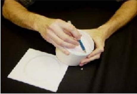
Next is to trim the silicone in the pvc pipe to allow us to remove the silicone from the pvc.
