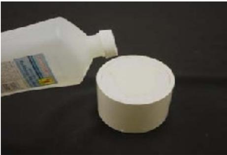
One trick of the trade is to use rubbing alcohol to help remove the silicone from the pvc pipe. The rubbing alcohol will make the silicone very slippery which aids in its release.
