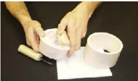
All that is left is to remove your original by flexing the silicone mold and removing your original.
