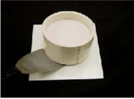
Allow the silicone to fully cure. The demold time of the High Strength 2 is approximately 12-18 hours. Once the silicone has cured remove the glue or clay that sealed the box to the base and begin to remove the mold from the box. Here we are using a putty knife to slide underneath the mold and the bulldog to break the glue off and remove it from the base.
