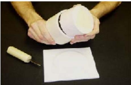
We then slide a dull knife around the outside of the mold which allows the rubbing alcohol to seep in and make the two very slippery allowing us to simply pull the mold out of the pvc.
