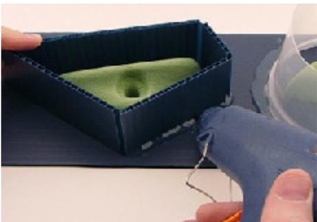
Seal the your mold boxes around the holds using hotmelt glue or modeling clay. Make sure it is a perfectly tight seal to contain the liquid rubber. If there is any gap in the mold box and the bottom, the silicone will leak out creating quite a mess and wasted silicone.
