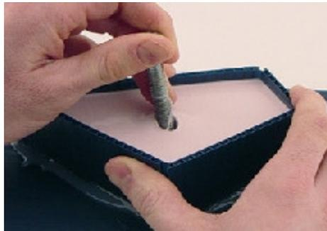
Once the silicone cures (overnight), remove the bolt from the cured silicone mold.
