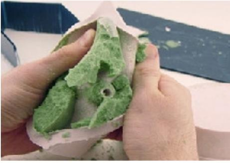
The last step is to remove the floral foam master. Because the foam is so fragile it will not come out in one piece. So just break out the bigger pieces and rub the mold with your hand to break any smaller pieces of the foam that are stuck in the mold. You now have beautiful rock climbing hand hold molds that will reproduce your exact foam hand hold out of resin. The texture and detail will be exact to your original!
