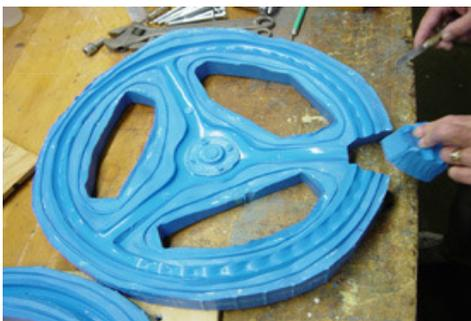
This piece will be inserted back into the mold immediately after the resin has been poured into the mold before it cures.
