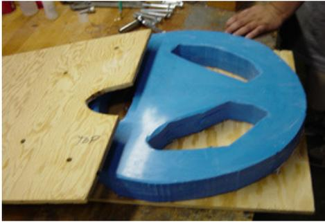
Using plywood, create a splint that will maintain the dimensional integrity of the mold and will make for easier handling of the mold while pouring. Two pieces of wood with holes drilled so bolts can hold it together work great.
