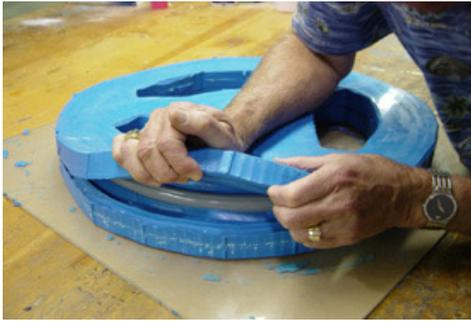
Slowly work the mold apart following the seam line between the two halves.
