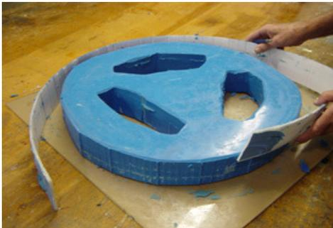
Once the second half of the mold rubber has cured, remove mold from the mold base, box, and inner box cavities.
