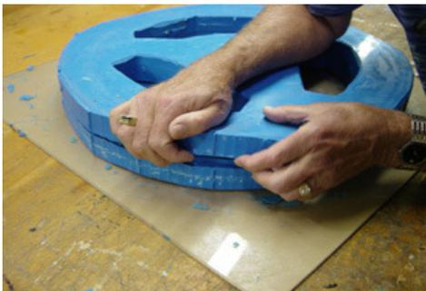
Find the seam line with your fingers and begin separating the two halves of the mold.
