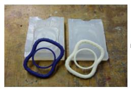
Remove the flash from the cast Flex 60 piece and you have a perfectly cast replica of your SLA original.
