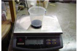
We are going to pressure cast this part using Alumilite's Flex 60 with blue dye added to it. The Flex 60 is a 1:1 urethane elastomer that cures to a 60A hardness that is similar to the hardness of car tire rubber. It has a 5 minute work time and a 1 hour demold time. So start by measuring out equal amounts of the Flex 60 A & B and then add Alumilite's Blue dye.
