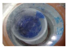
Using a vacuum chamber and pump, degas the Flex 60 to remove all of the mixed in air.
