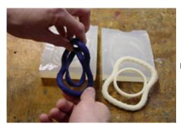
Notice the flexibility demonstrated in the cured Flex 60 casting.
