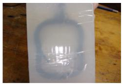
Observe the resin flow through the mold until it is completely filled.
