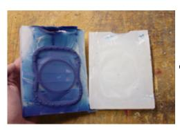
Once cured, remove from the pressure tank and open the mold.
