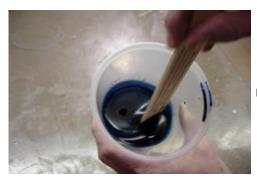
Mix the material thoroughly. Be sure to scrape the sides and the bottom well.
