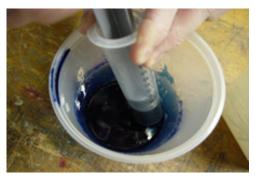
Using a large plastic syringe (found at local medical supply companies), suck up the degassed Flex 60 into the syringe which will allow you to inject the resin into the mold rather than trying to pour it.
