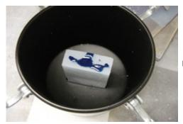
Fill the reservoir completely and place the entire mold into your Alumilite Pressure Pot.
