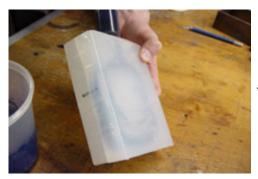
Tilt the mold if necessary to flush air pockets out of trapped areas of the mold.
