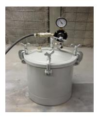
Fill the pressure pot with 40 psi and allow the part to cure under pressure (approximately 30-60 minutes depending on mass).
