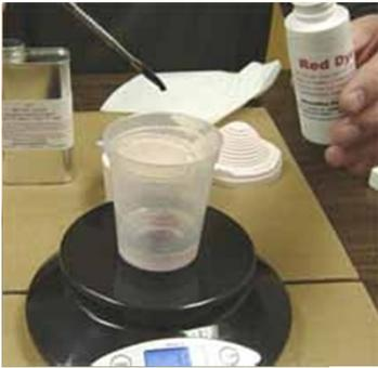
After you measure out the A side, add a few small drops of dye to color the resin. Here we will add a few extra drops of red to help differentiate resin in the pictures.
