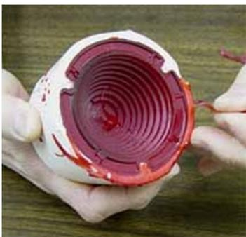
It is often times easier to remove the flash while the part is still in the mold. Simply peel it away from the seam line and throw it away.
