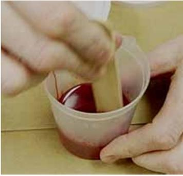
Put your stir stick down to the bottom of the container and stir the resin extremely slow for 2 minutes. This will drastically reduce the amount of air bubbles you create as you mix seeing as though we will not be using equipment to help us eliminate bubbles in our casting.
