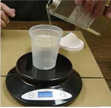
Measure equal amounts of A and B. Shown in this picture is an inexpensive digital kitchen scale Alumilite sells that is perfect for measuring silicone rubber and resin.
