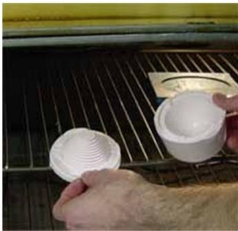
The first step to casting your tail light lense is to warm your mold to help the resin cure properly in thinner sections. We recommend 15-30 minutes at 150 F or 1 minute/lb of rubber on high in a microwave. This will make the molds warm to the touch but should not be so warm that you can not hold onto them.
