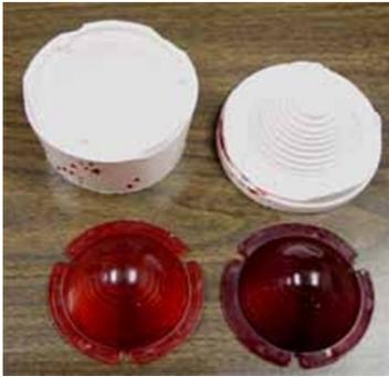
Here you can see the original lense (left), along with the two piece rubber mold (top), and the darker cast reproduction (right). As you can see our cast replica is darker than the original. If you wish to match an exact color, simply run small test batches to figure out the exact amount of dye you need to match the color you desire. Then cast your piece with that amount of dye added to the Water Clear.
