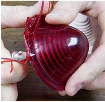
The other option is to simply pull the part out of the mold and trim it off with an Exacto knife.
