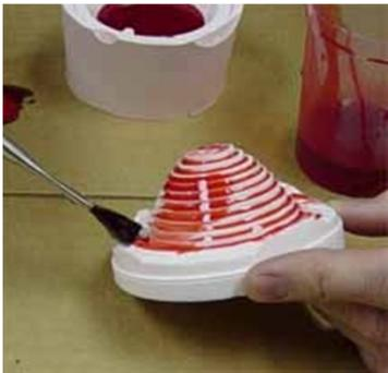
Next, paint the remaining resin onto the male portion of the rubber mold. This will reduce the surface tension from that half of the mold and help the air bubbles migrate to the seam line and out of the casting.
