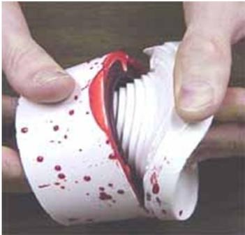
Once the resin has cured, separate the two halves of the rubber mold.
