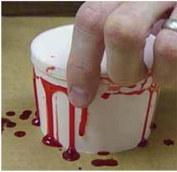
Simply lay the top half on the bottom and do not push it down. Make sure the locators and mold are in the proper place. Then walk away from it. Let the mold sit for a minimum of 2 hours. If your part is thinner than 1/8", it is recommended to post cure the part in an oven at 150 F for 30-60 minutes to help the thin resin piece to cure properly. Allow the mold to cool before demolding.
