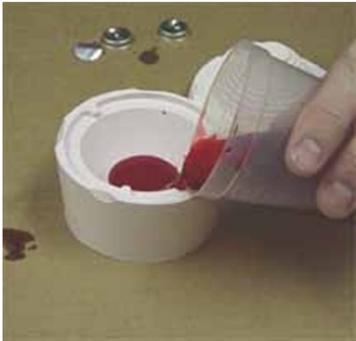
Start by pouring some of the resin down the side of the mold very slowly. Fill the mold up approximately 1/2 way.
