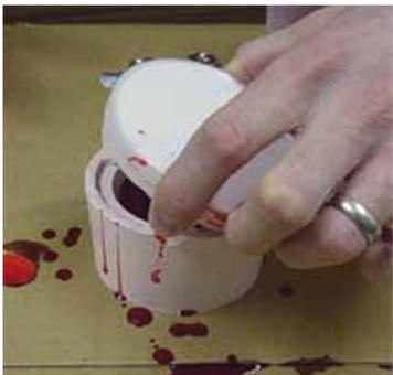
After you've painted some resin on the male half of the mold, line up the locators and on an angle, slowly lay the male half onto the female. This will allow the air to be squished out the seam and reduce the amount of air that will be trapped.
