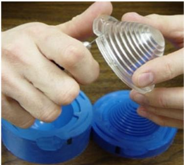
Use an Exacto knife to remove any flash. It is also a good idea to remove any flash that is left on the mold surface before starting the process over. The left over flash may make your parting line bigger and may even distort your part if it is not removed.
