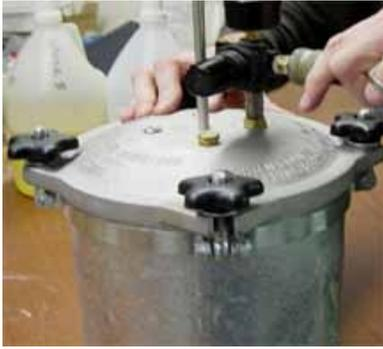
**SAFETY: MAKE SURE YOUR POT IS RATED FOR AT LEAST 30-40 PSI AND MAKE SURE THERE IS A SAFETY RELEASE VALVE IN PLACE SO THAT YOUR POT NEVER TAKES IN MORE AIR PRESSURE THAN WHAT IT IS RATED FOR.** Then connect your air source making sure your regulator is set for 40-50 psi. If you have a small compressor it may be a good idea to have the air compressor filled with air so it doesn't take too long to fill the tank with the required pressure.
