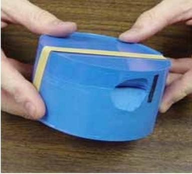
Use a rubber band or tape to hold the mold together in place. Do not over tighten to prevent distorting the rubber and your part. Simply hold it together so the locators prevent the two halves from sliding or separating.
