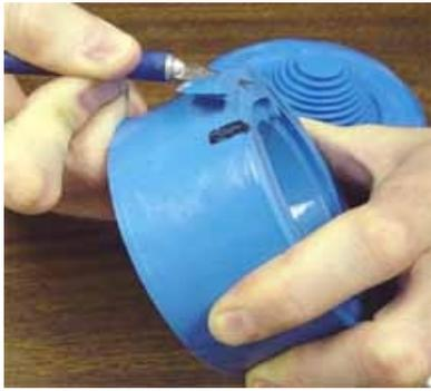
Now you are ready to cut your pour hole in the rubber mold. Take one half of the rubber mold and cut a channel that will act as the pour hole and reservoir for the resin to fill the mold. Cut it on an angle so you only have a small slit that is in contact with the part and a bigger area where you will pour the resin.
