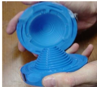
Then separate the mold. The lense is actually on the male half of the mold (the one closest to the bottom of the picture in the person's left hand).
