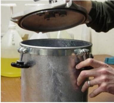
Wait approximately 2-3 hours (depending on the mass of the part being cast and mold temperature) and remove the air pressure from your pot. Then remove the lid.
