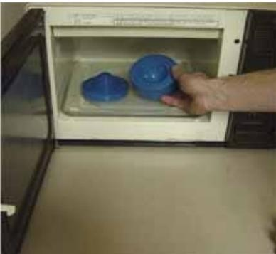
The first thing you will want to do is preheat your mold. You can either place your mold in a microwave for 1 minute on high per lb of rubber or place the mold in a conventional oven at 150 F for 15 minutes. The mold should be warm to the touch but not so hot that you can not hold onto it.
