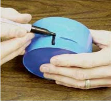
The next thing we suggest doing is to use a permanent marker to draw a line that will help you visually line up the mold much quicker than trying to match up the locators you cut in the rubber every time you need to put the mold back together.
