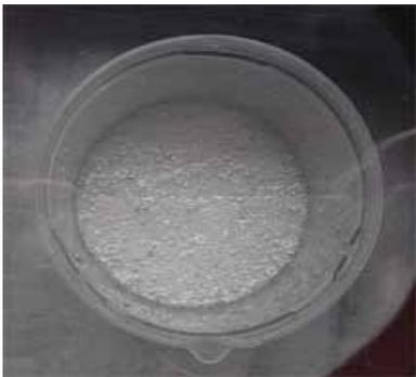
Watch the material rise in volume and then collapse. Once the material collapses, you have removed 98% of all the air you mixed in. Allow the resin to vacuum for another 30 seconds (as long as you are not closing in on the 15 minute gel time).
