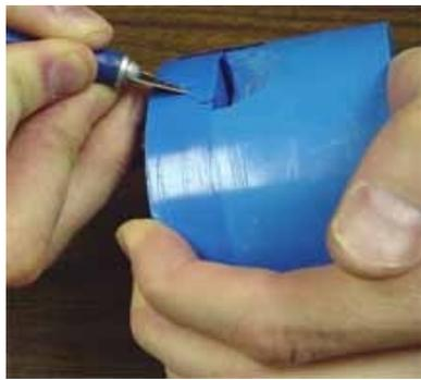
Now cut the other half the same way. This will create a nice reservoir to hold the extra resin needed for pressure casting to make sure you do not have a short pour.
