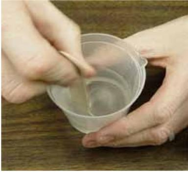
Stir the resin thoroughly until absolutely no swirls are seen. Be sure to scrape the sides and bottom well.
