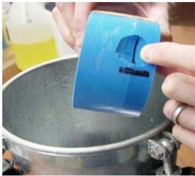
Take your mold out of the pot and touch the resin in the reservoir to make sure it has fully cured. (Because the resin is Water Clear, it is difficult to see the casting in the next few pictures.)
