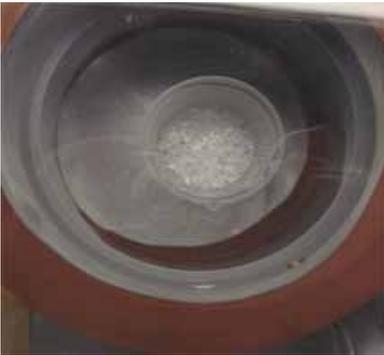
Place the mixed Water Clear resin in the vacuum chamber and turn on the pump.
