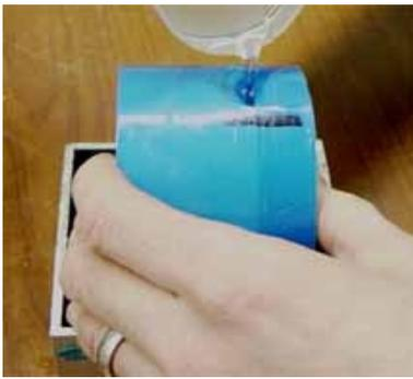
Then stand the mold upright again and continue pouring the mold until you have filled the mold and the entire reservoir.
