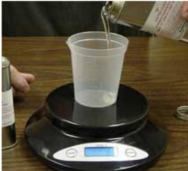
Measure equal amounts by weight of A & B of Alumilite's Water Clear. Use a container much bigger than needed to hold the resin due to the fact that it will expand as you vacuum it similar to the mold making rubber.
