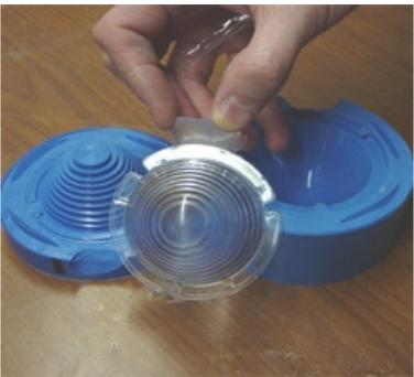
Here you can see some of the flash along with the resin that cured in the pour hole/reservoir that the person is holding onto.
