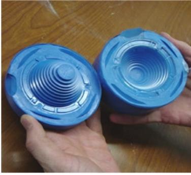
If the mold or part is still warm, you may wish to leave the mold open for 10 minutes to cool. As the cast piece cools, it will harden.
