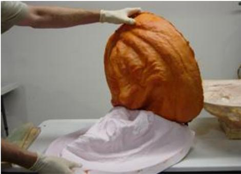
Peel the rubber mold off of the Skin Coat piece to demold.
