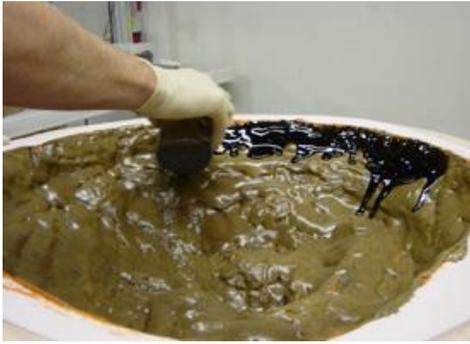
If you have thin areas of foam, mix up a smaller second batch and concentrate brushing the material on the top edge and in the thin areas. Then allow it to expand and cure.
