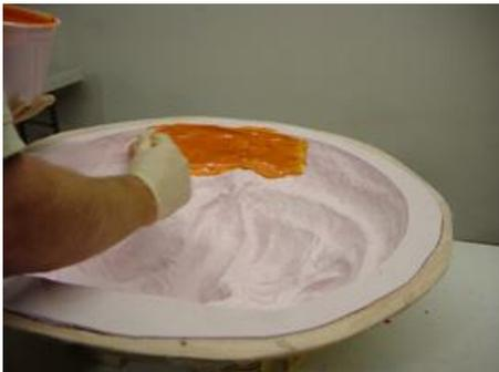
Mix equal amounts of Alumilite's Shell Casting Resin and add a small amount of orange dye. As soon as you the two liquids come in contact they will begin to gel. Mix thoroughly for 1 minute and then begin to spread/paint the Skin Coat into the mold. Only mix what you can apply within the 7 minute open time of Shell.
