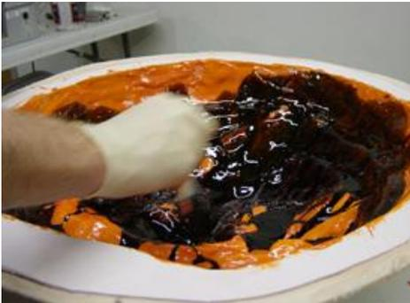
Using a cheap paint brush (will not be able to salvage), spread the mixed foam throughout the mold until it is all covered.
