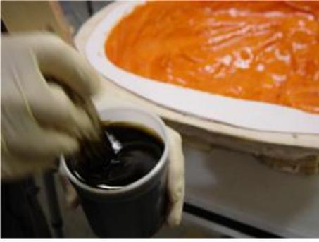
An easy way to build up thickness with out using a ton of Shell is to brush in a layer of Alumilite's 610 Foam. The 610 Foam will add reinforcement as well as wall thickness to the piece. Here we have used approximately 8 oz of A + 8 oz of B of the 610 Foam with a small amount of Brown Dye. Using the brown dye in the foam will give the original orange outside layer a little bit of depth.
