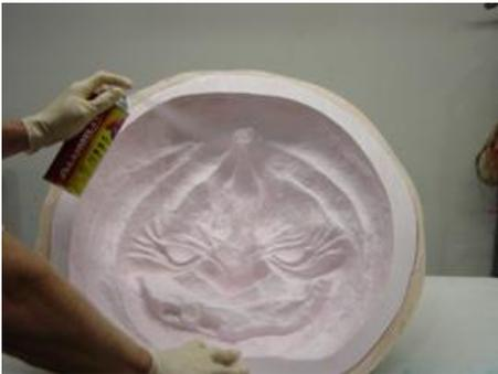
Set the rubber mold back into the mother mold and make sure the locators are all pushed in place in the mother mold. Then be sure to spray in Alumilite's UMR in to the mold. Although it is not necessary, the UMR will aid in the release and help to preserve the life expectancy of the mold.
