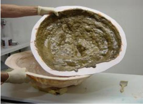
Once the 610 Foam has expanded and cured, remove the rubber mold from the mother mold and prepare to remove your reproduction.
