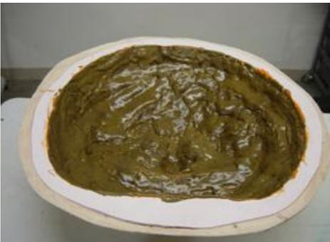
Continue to brush the foam up the walls until it begins to expand. Then allow the foam to expand and cure.
