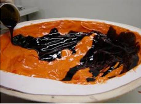
Pour a small amount of the thoroughly mixed 610 Foam along the top edge and allow it to flow down.
