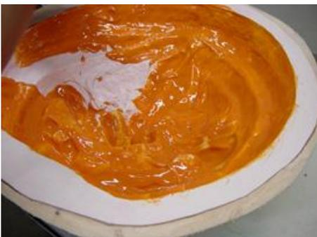
Continue until the entire mold cavity is evenly coated. Try to build a minimum of 1/16-1/8" thick layer throughout the mold.
