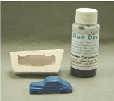
Once your Alumilite resin has cured, demold your cast piece. Your dyed cast replica will have the exact detail of your original.
