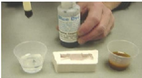
Next, following mixing directions for your resin, measure out resin (enough to cast your part). If using 1 oz bottles of dye, squeeze out desired drops into the "A" side of the resin. If using larger bottles of resin, either transfer a drop(s) from a stir stick, or weigh out desired amount of dye. Stir the dye into the 'A' side thoroughly until uniform color is reached.
