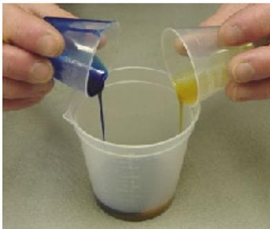
Pour both sides of the resin into a cup. Stir until a uniform color is reached (about 25 seconds).
