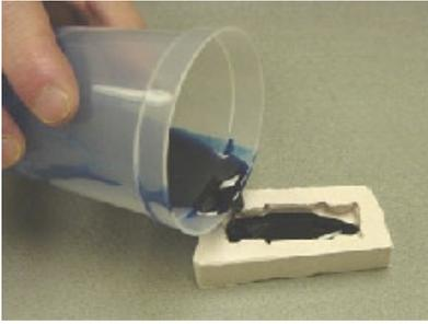
Slowly pour resin into your mold. Tipping the mold a little while you pour will help fill in any undercuts and reduce the chance of air bubbles. Use resin in accordance to open time and demold time.
