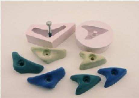
Picking up where we left off from making our own rock climbing hand hold molds, we'll now walk you through how to cast them. We have two different types of molds, first the a standard mold with a silicone stem and secondly a mold where we use the actual bolt to act as the stem to our hold.
