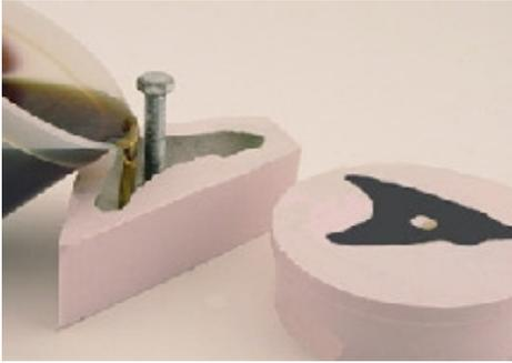
Once the resin is mixed thoroughly, pour the resin into your molds. On the right you can see the mold that is using a silicone stem and the mold on the left has the bolt as the stem.
