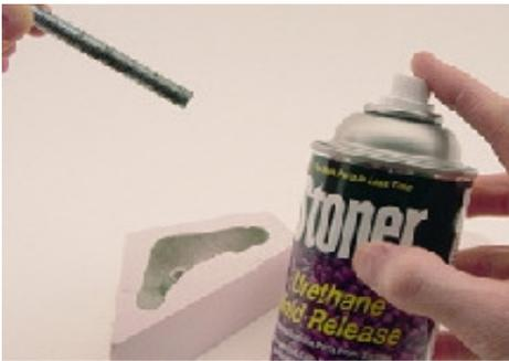
If you are going to use a bolt for the stem it is very important that you mold release the bolt. Alumilite's casting resins will bond to metal unless it is mold released. We use Stoner Urethane Mold Release which works exceptionally well for making sure the bolt releases from the casting.
