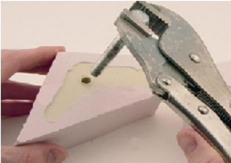
Shortly after the resin changes color, remove the bolt with a pair of vice grips or pliers. I would recommend doing this within a minute or two of the resin changing color. If you wait too long, you will have to unscrew the bolt.
