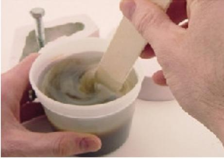
The next step is to mix Alumilite casting resin. The mix ratios of most of our resins are 1:1 by weight or by volume. Mix the resins thoroughly until no swirls are left in the mix container. The resins are non toxic and very easy to use. They mix and pour like water making them extremely user friendly. Mix the resin thoroughly for 20-30 seconds.
