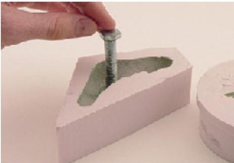
Insert the bolt back into the stem hole after it has been sprayed with mold release.
